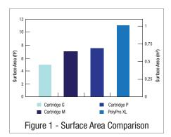
Surface area dictates just how long a filter will last and how it will perform. However, increasing surface area without considering the flow path between the media's pleats could result in flow restrictions and early media blinding. To achieve the optimum between surface area and performance, CUNO has designed PolyPro XL so that the pleating process and media support materials work together to provide enhanced flow characteristics and longer service life.
